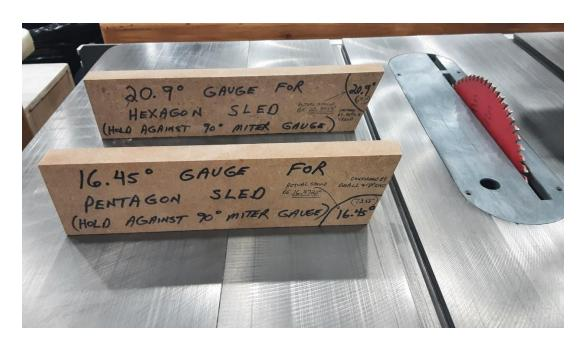
I find the best method is to first set the blade angles using the blade blocks first. The best way to do this is to hold it against your miter gauge set at 90 degrees to ensure an accurate reading against the body of the blade raised to its highest level. I typically put a light behind the blade so that, as I stare down the length of the blade, I can more easily see any gap between the setup gauge and the blade body. **Don't forget to unplug your table saw before doing this!!**
