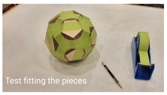
If all the pieces fit properly, remove the marked temporary tape sections, lay the 3 separate sections out flat again, then apply glue to both faces of just the facets being joined at that time. I would use one of two procedures here depending on what type of glue I intend to use and whether or not I have enough band clamps and/or #107 rubber bands (7" x 5/8") available:
