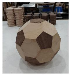
To verify that you cut the pieces to the correct size for what will end up as a regulation size 5 soccer ball after turning (between 8.6" and 9.0" in diameter), the dimension of the rough ball at this point (measured from the *flat side* of opposing hexagons) should be approximately 8.8" or so – assuming you made your hexagons and pentagons about 49mm on each facet. Mine end up about 8.88".
