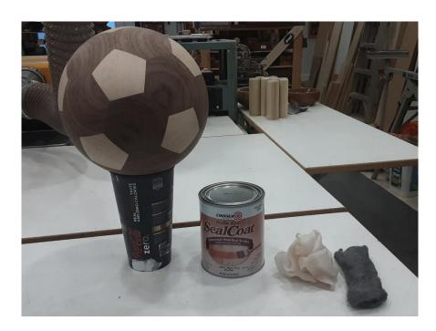
Then I spray on multiple coats of satin spray lacquer (I use Deft, Minwax or Watco, depending on what is available locally). To do this on a round ball of this size, I simply set it on a tall plastic cup on a turntable and spin it as I spray.
