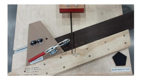
Successive cuts are completed on the small piece that has been cut off the main board by then rotating the piece clockwise until all sides are cut.
