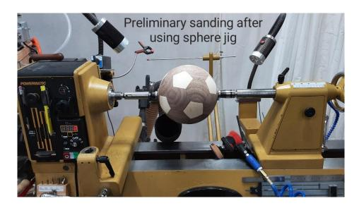
Once the preliminary sanding is done, assess which joints need to be filled. Don't bother filling any joints before this since some of the gaps that may have appeared initially will disappear as you turn away the outer rough surface of the ball. It is only worthwhile doing this once you are done turning, sphere jigging and preliminary sanding.
