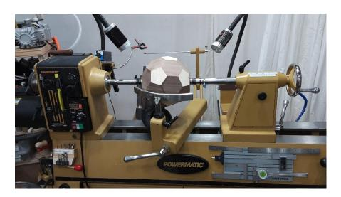
If you <u>will not</u> be using a sphere jig, turn the ball as round as you can using a bowl gouge or carbide tool, leaving a nub about 1/8" high near each steb center that you will turn off later. **Use a turning speed of just under 1000 rpms.**
