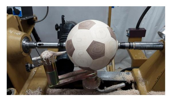
Then do your preliminary sanding. I use a pneumatic random orbit sander and start at 120 grit to remove the very small "grooves" left by the cutter on the sphere jig, using a turning speed of around 500 rpms.
