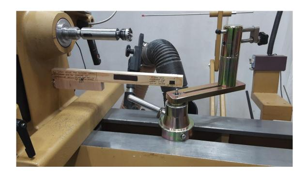
10.Next complete the rounding of the ball with the sphere jig to a diameter of *at least* 8.65". This will leave enough material that will be removed in final sanding such that the ultimate result will be the desired finished diameter of no less than 8.6" (but as much as 9.0" if you want to stay within the regulations...).
