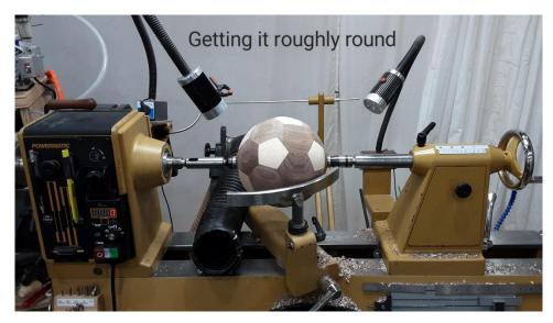
Then carefully set up your sphere jig to ensure it is perfectly centered on the ball. This can be complicated so I use a guide stick to set the sphere jig at the correct distance off the headstock.
