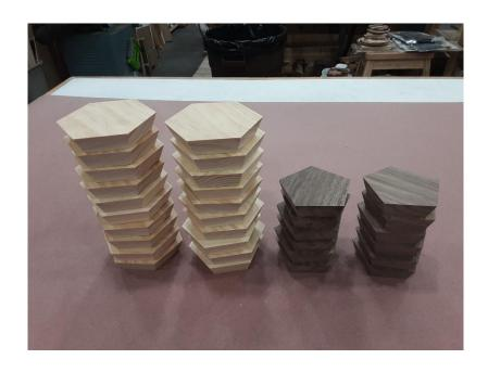
7. Next you should do a dry assembly to verify the correctness of your cuts. I use Scotch Rough Surface Painter's Tape for this since it is easier to work with than standard masking tape. I use the 1.41" width tape rather than the 1.88" so that you can still see both edges of the joint to tell if either end has a gap. I do *NOT* use blue painter's tape since it isn't "sticky" enough to hold the pieces together well enough during the glue-up phase.
