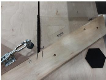
CNC-cut templates for pentagons, hexagons and octagons are also available from Amazon in addition to the usual squares and triangles (usually found by searching for quilting templates in those shapes). They make the setup of the fences on these jigs quick, easy and crazy accurate.
