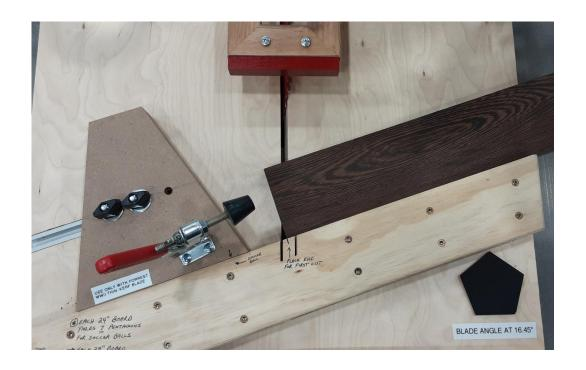
The board then gets flipped and clamped against the adjustable stop.
