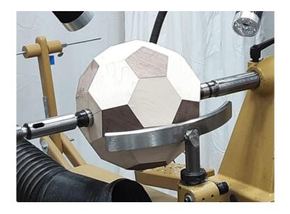
So, if done correctly, all the marks left on the hexagons by the steb centers will be turned away when the nubs are removed or sanded away in the final finishing process, resulting in an unmarked final surface.
