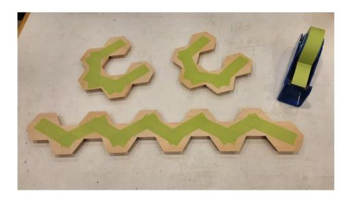
At this point, you may want to put numbers on the outside edges of each of the 10 hexagons in the zig-zag pattern to facilitate the later installation of band clamps. Here is what it looks like after glue-up – forgot to take a picture of it prior to that – sorry....
