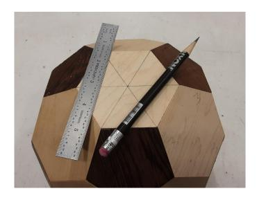
Then mount the ball on the lathe using safety (steb) centers so that there are no deep depressions made into the mounting surfaces (standard centers will likely leave point holes deeper than you will turn away, meaning you would have to fill them – and those fills will be rather
